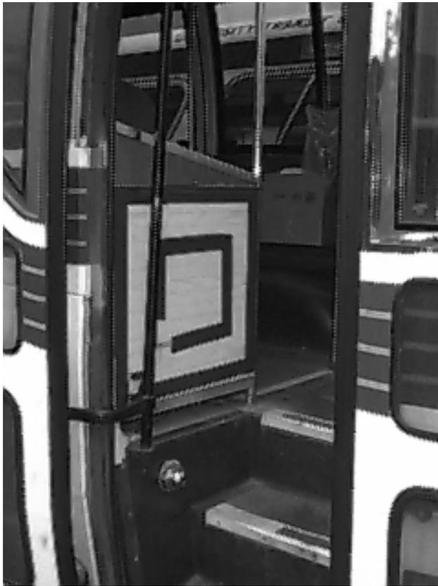
**FIGURE 4 Front RF antenna mounted to bus**
