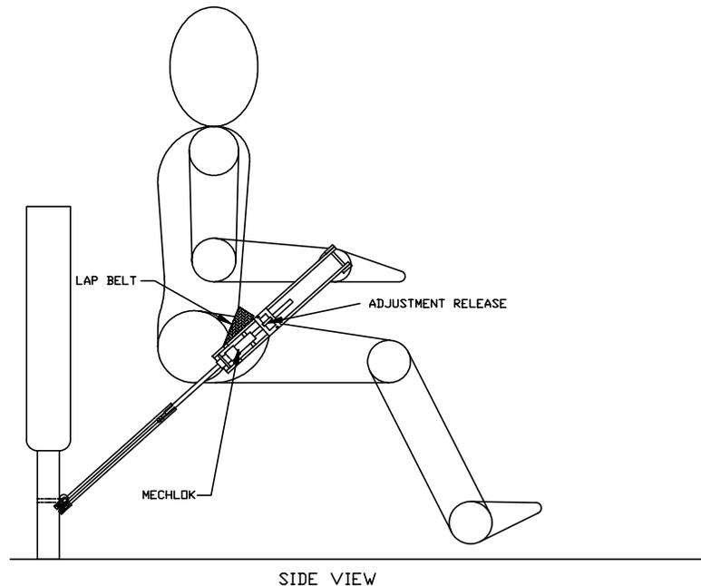
**Figure 1. Design concept for restraint system**
