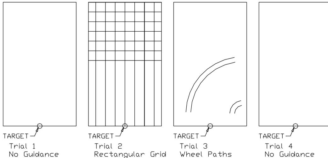
**Figure 3. Floor patterns to assist with wheelchair positioning.**
