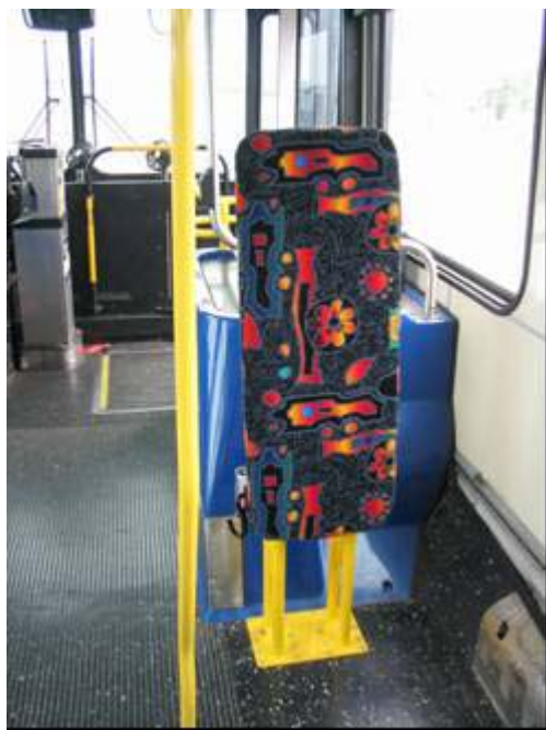
FIGURE 3 - A rear-facing securement station on a BC Transit vehicles showing the padded backrest and aisle side stanchion.
