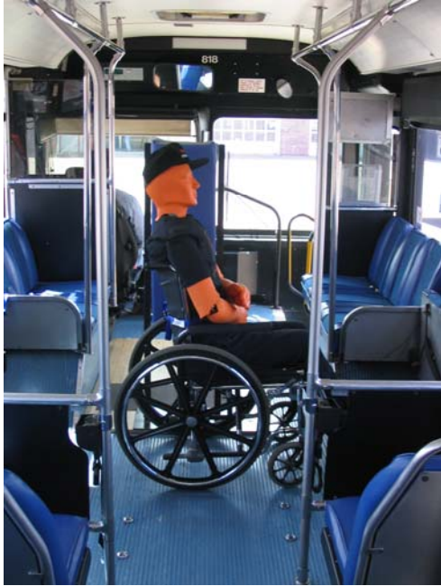
FIGURE 19 – The results of a panic stop when a manual wheelchair occupied by a test dummy is side facing and has only a forward wall for “Securement.” The manual chair did not move appreciably during the actual stop (left) but it tipped over on its side during the forward acceleration due to the bus suspension system rebound (right).(LTD vehicle)
