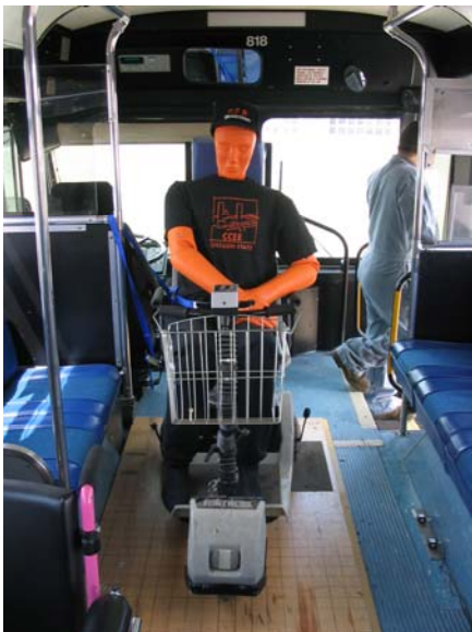
FIGURE 17 – Test dummy in Three-Wheel Scooter backed against rear-facing securement backstop mounted in center aisle of LTD bus.
