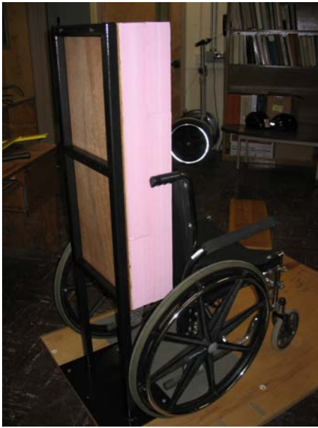
FIGURE 16 – Construction of the backrest used in rear facing Securement tests. A steel frame was built and welded to a base plate. The wheelchair contact plane is moved away from the frame using foam to allow lower portions of the wheelchair to fit.
