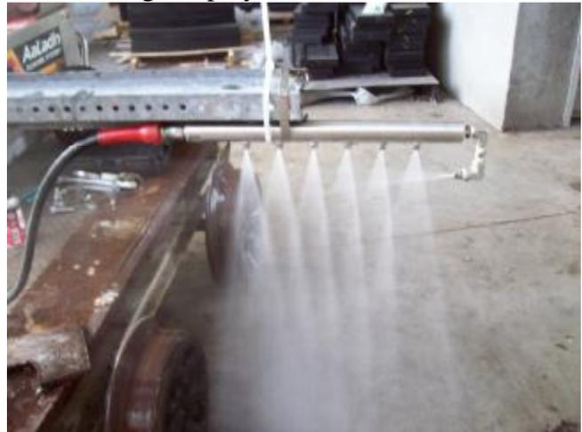
Fig 2. Spray bar with 7 nozzles for pressure washing
