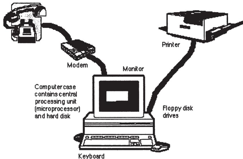
Figure 4.1 Hardware Components of a Personal Computer.
