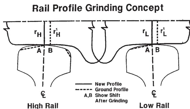
**Ground Contours of High and Low Rails Shift Point of Wheel Contact from A to B, Increasing Differential Rolling Radius to an Extent Making Wheelset Self-Steering on Curves Up to Somewhat Over Two Degrees of Curvature. Gauge Corner of High Rail is also Relieved Slightly to Avoid Contact with Flange Throat.**
