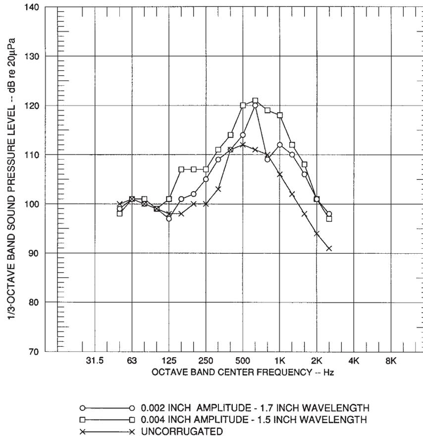
**FIGURE 8-6 EFFECT OF CORRUGATION AMPLITUDE ON WHEEL/RAIL NOISE**
