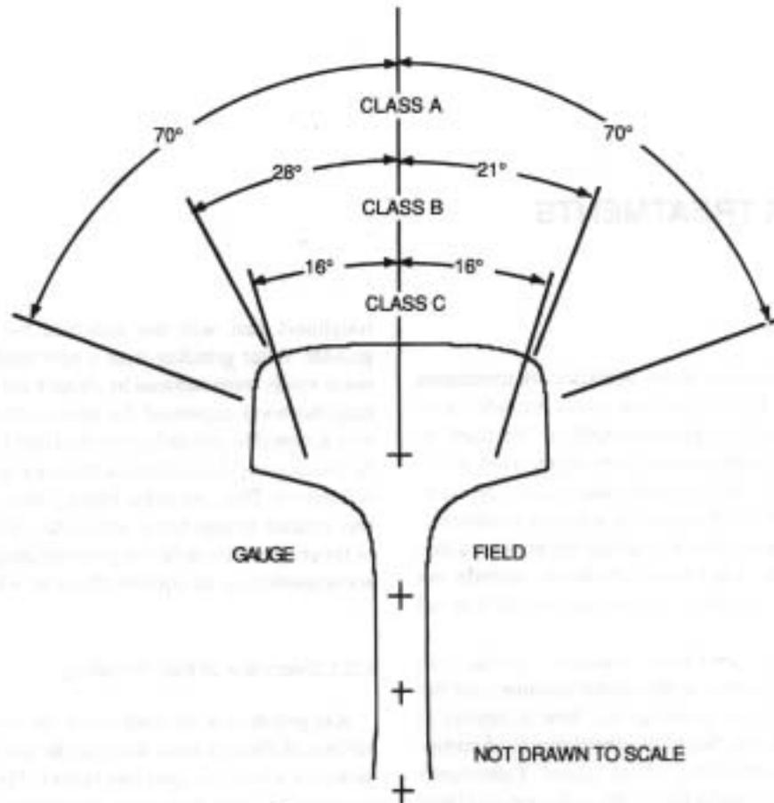
**FIGURE 8-1 RANGE OF MOTOR ANGLES FOR DIFFERENT EQUIPMENT CLASSES (ZETA-TECH, INC.)**
