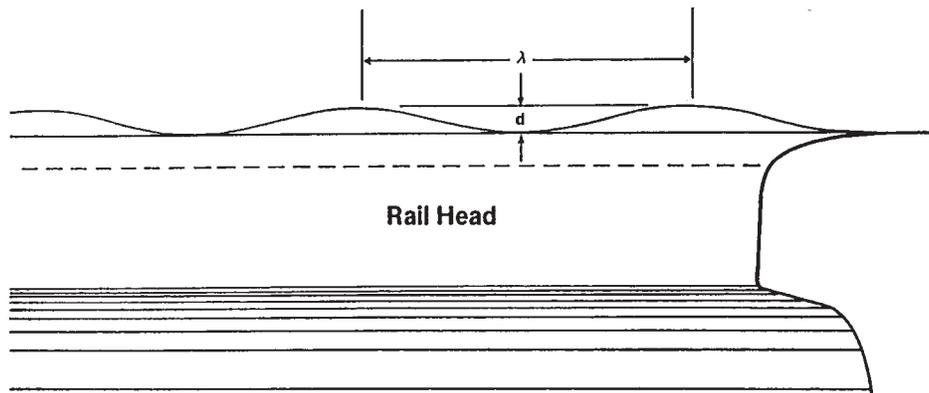
**FIGURE 8-3 RAIL GRINDING WAVELENGTH**
