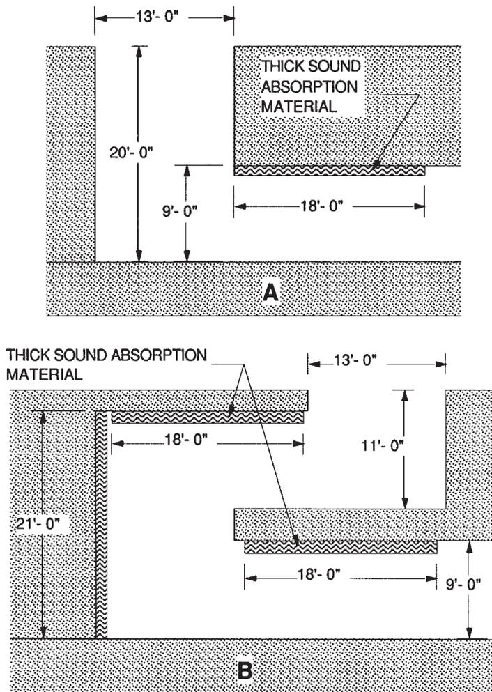
FIGURE 9-11 TYPICAL BEND IN SHAFT
