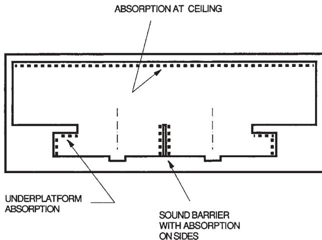
**FIGURE 9-3** ACOUSTICAL TREATMENT OF STATION PLATFORM AREAS
