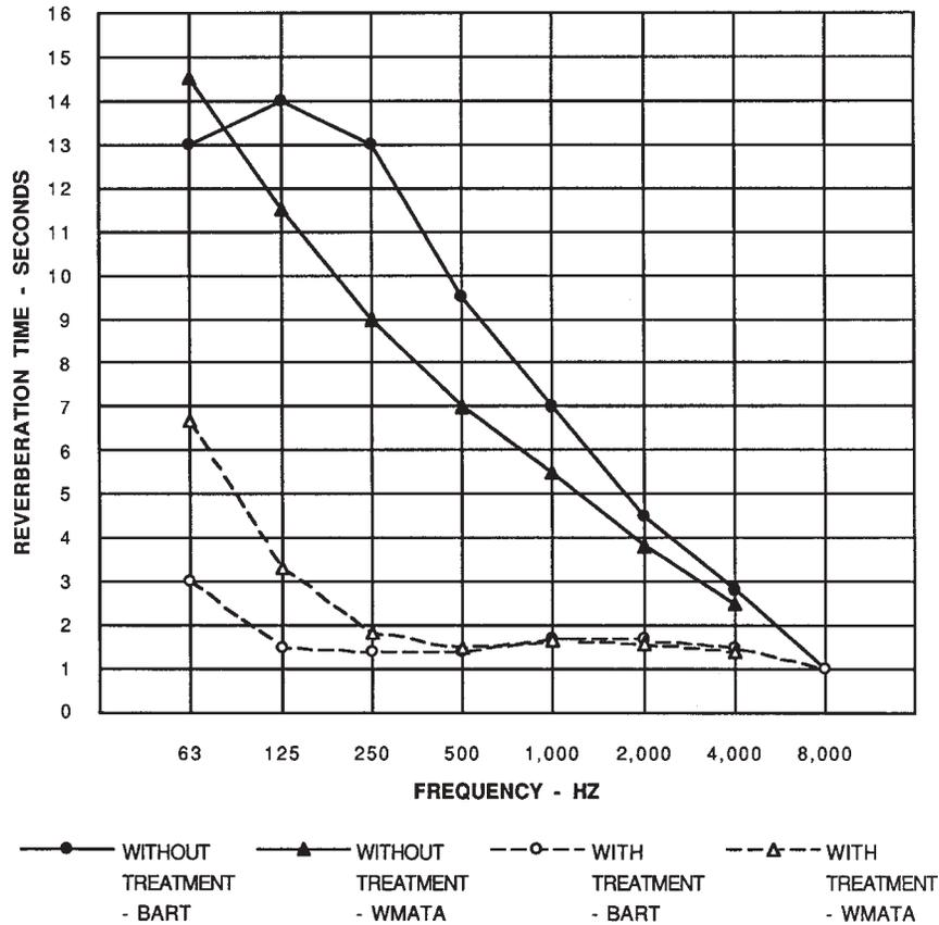
**FIGURE 9-4 REVERBERATION TIMES FOR TREATED AND UNTREATED STATIONS**
