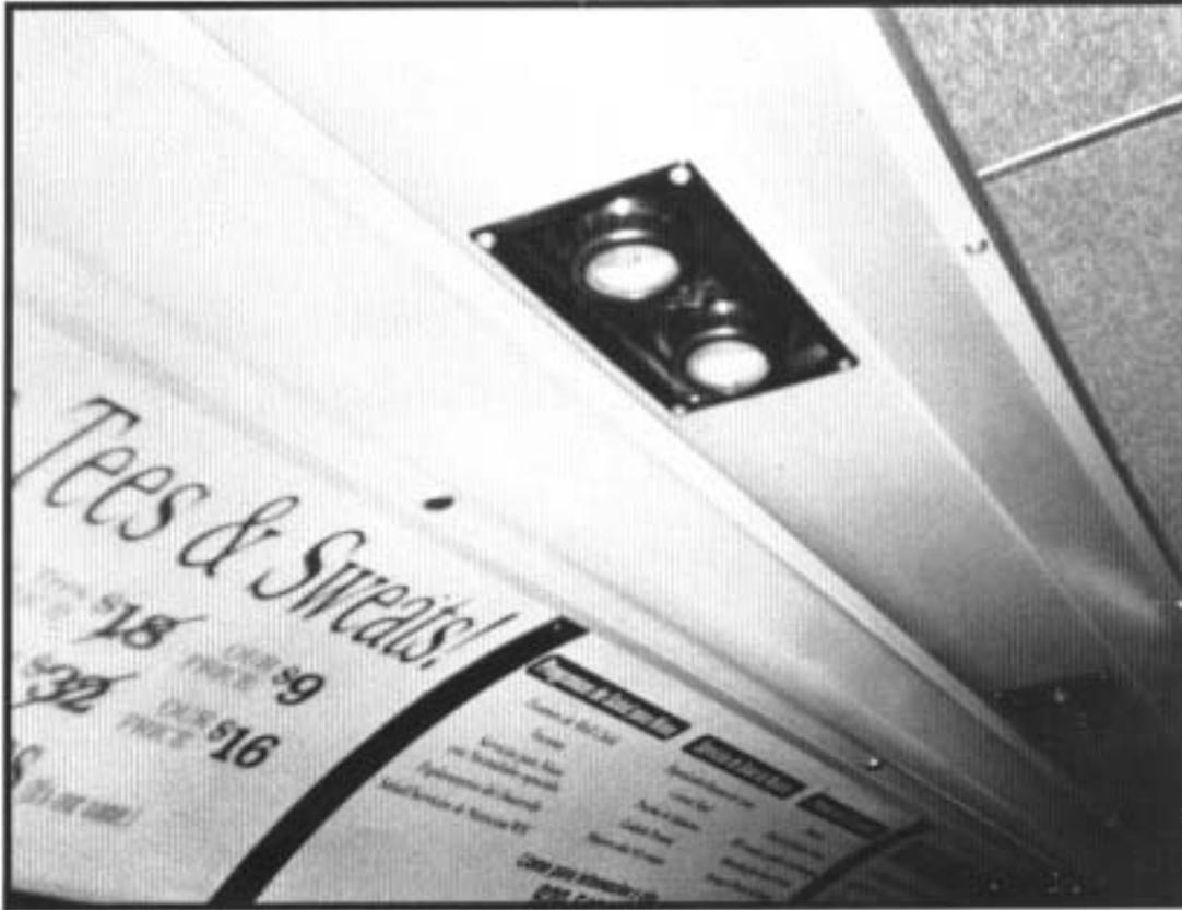
Figure 5. New Neoplan bus with passenger reading lights.
