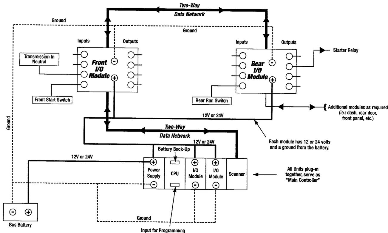
**Figure 4-3** Schematic showing how multiplexing uses its own data network and the battery's power and ground current to control the engine starting circuit
