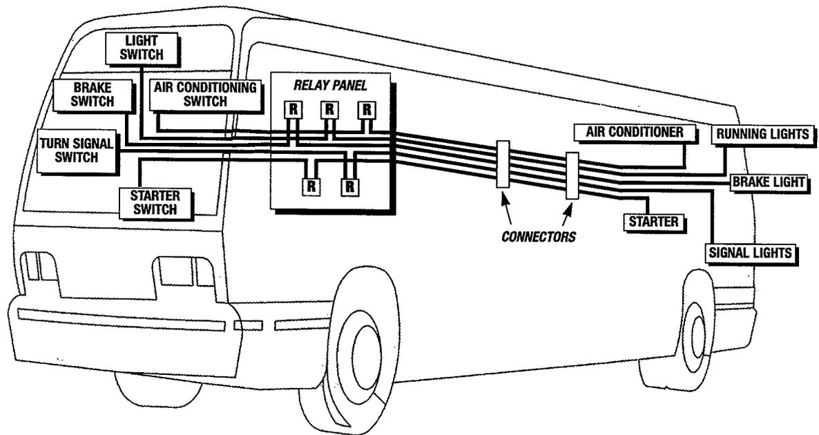
**Figure 4-1** Traditional "hardwired" electrical system with separate wires connecting switches, relays, and electrical devices.
