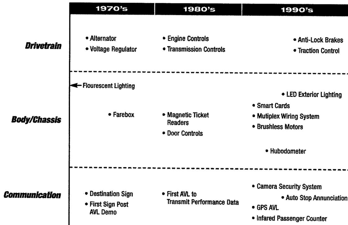
Figure 1-1 Evolution of bus electronics during the last three decades.
