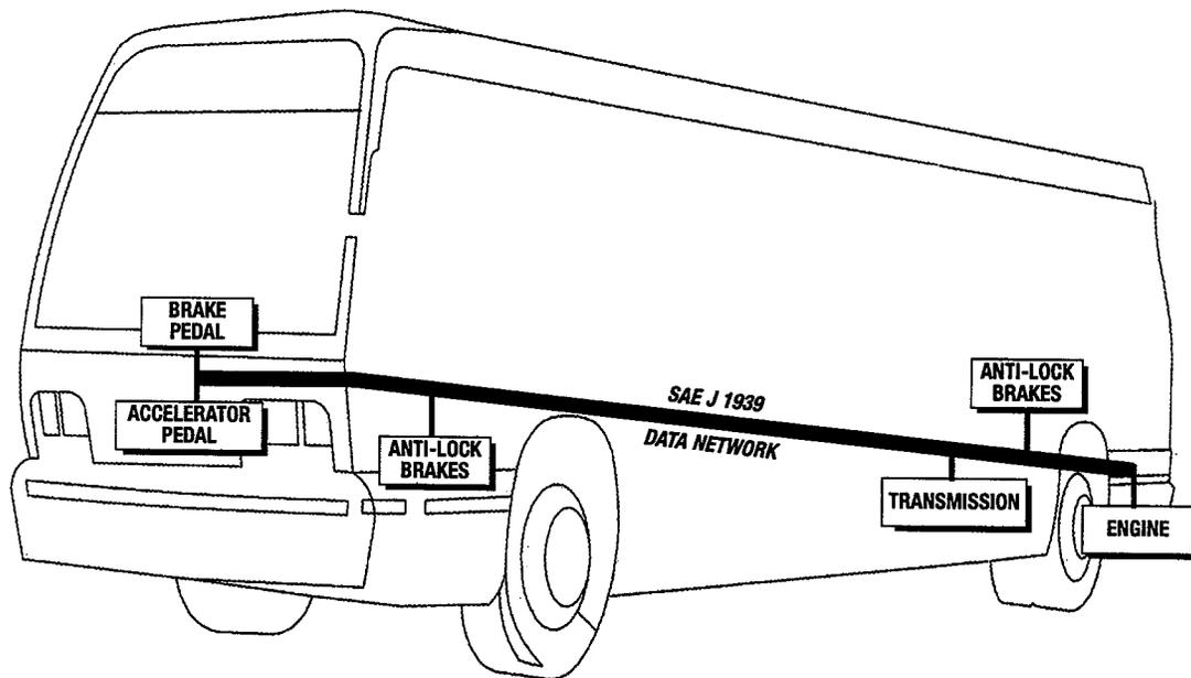
**Figure 5-2** Drivetrain integration achieved through SAE J1939.
