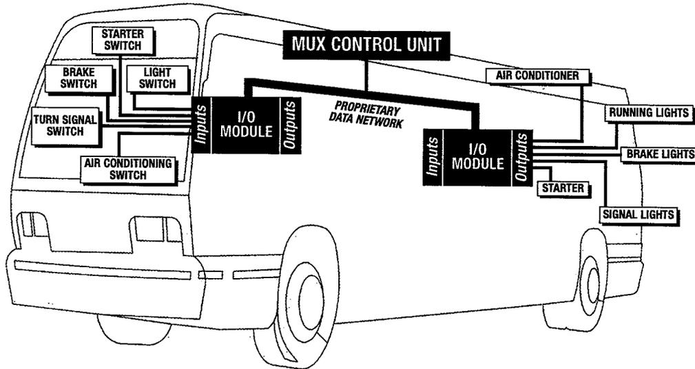
**Figure 4-2** *Instead of running individual wires to each device, multiplexing uses a controller and satellite modules to control several functions over its own data network.*
