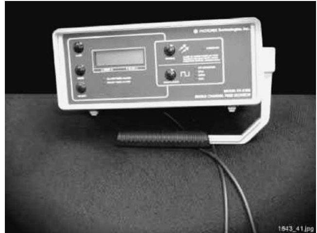
Figure 3. Front view of Photonix fiber-optic unit.
