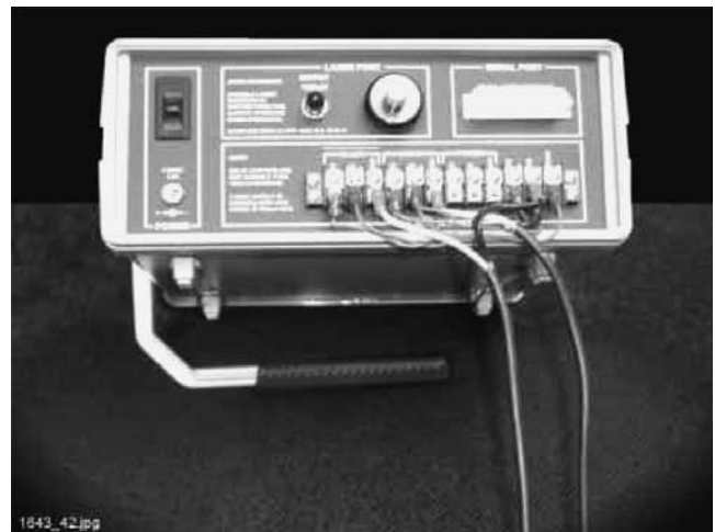
Figure 4. Back side of Photonix detection system, showing output relay control connections for major and minor trigger alarms and fiber-optic input and output ports.
