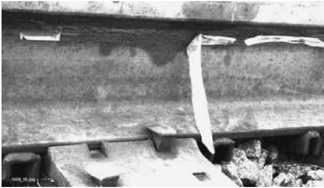
Figure 1. Fiber-optic strand protected by epoxy and tape on the rail.
