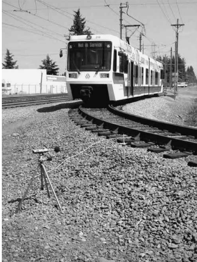
Figure 2. Test site and typical Portland Tri-Met car.
