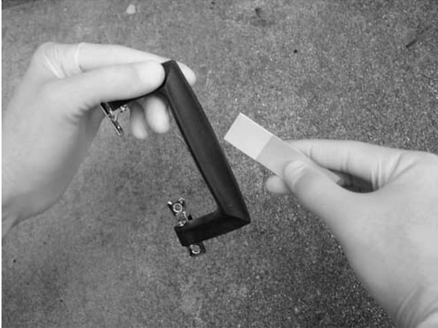
Figure 10. Dry transfer strip contaminating a handle.
