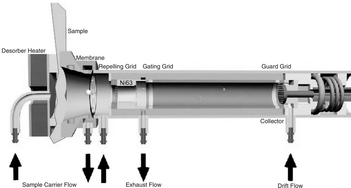
Figure 6. IMS process of tested device.
