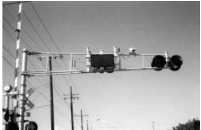
*Figure A-5. Overhead LED blank-out sign with warning flasher and CCTV for data recording.*
