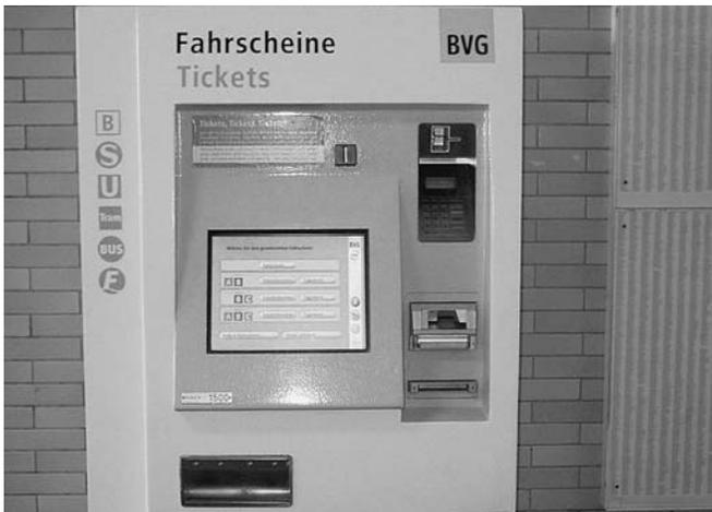
**Figure 7** Upgraded ticketing machine for dispensing proximity smart cards in Berlin.
