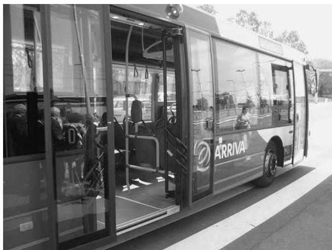
**Figure 6** A low-floor bus with wheelchair ramp access in Amsterdam.
