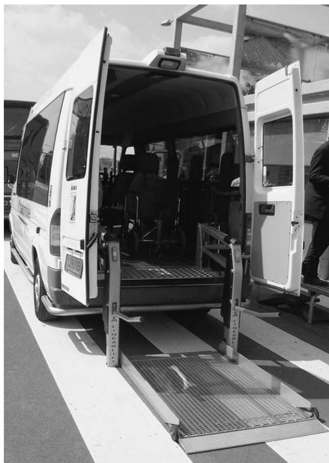
**Figure 7** Extended wheelchair lift on a Stadsmobiel bus, part of Amsterdam's special transportation services program.
