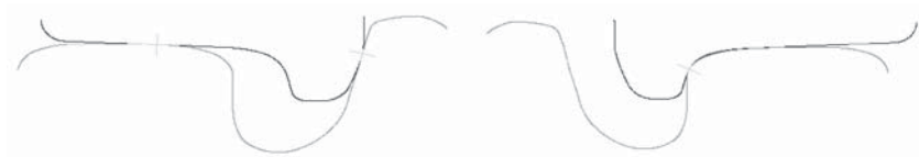
(c) Flangeway width 1.613 in. (optimal).
