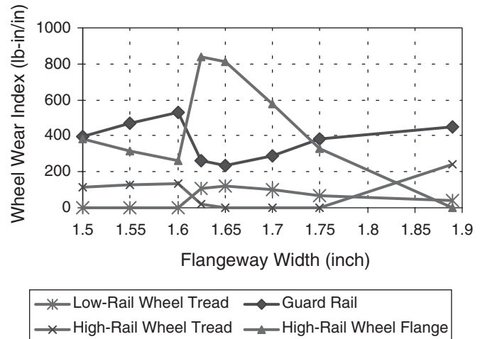
Figure 21 Guard rail W/R wear, wheel flange angle = 75 degrees, AOA = 58 mrad.
