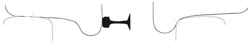
Figure 59 Restraining rail W/R animation, wheel flange angle = 63 degrees, AOA = 20 mrad, restraining rail height = -0.23 in., flangeway width = 2.73 in.
