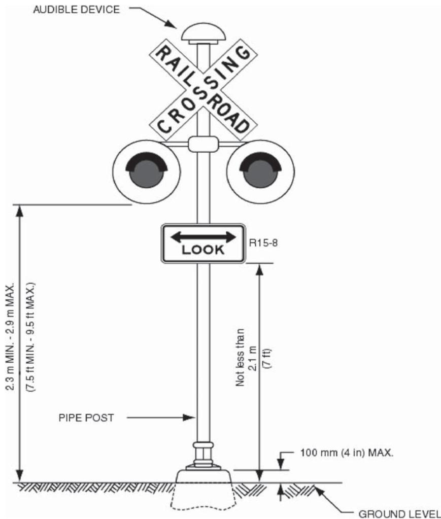
**Figure 4** LRT Flashing-Light Signal Assembly for Pedestrian Crossings.
