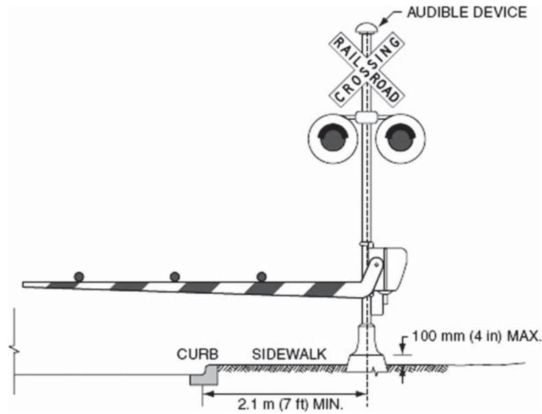
**Figure 1** Pedestrian Gate Placement Behind the Sidewalk.
