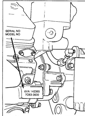
FIGURE 3 Location of DDC engine serial and model numbers (6V-71 shown). (Source: Detroit Diesel Corporation)
