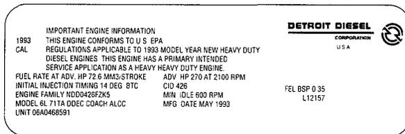
FIGURE 2 DDC engine certification label. (Source: Detroit Diesel Corporation)
