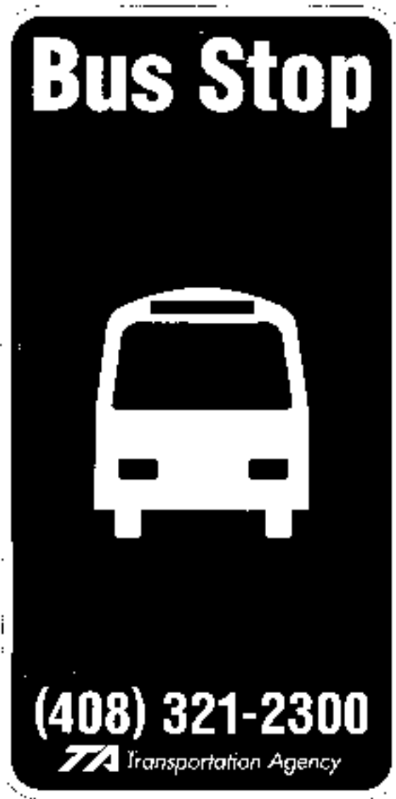
Santa Clara County Transportation Agency bus stop sign without route identifier. This sign is placed at stops serving one route.
