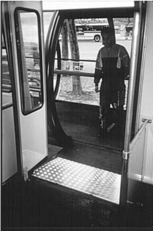
Figure 6-15. The Halmstad technology was refined with the use of a simple bridge in the Curitiba bus system in Brazil.
