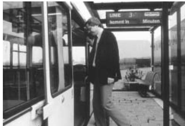
Figure 6-16. Two-sided guidance allowed precise docking at platforms, a key goal of the bus rapid transit concept.
