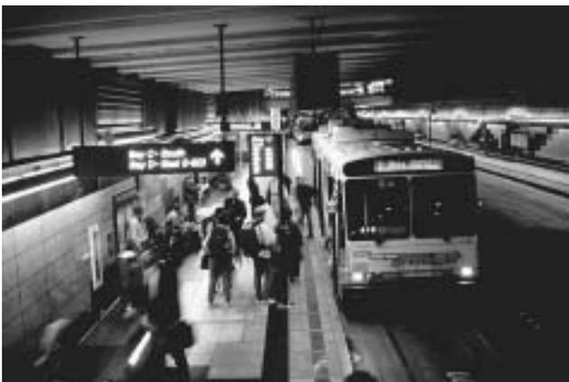
Figure 6-17. The Seattle Metro operates a dual-propulsion, articulated bus from Seattle’s downtown tunnel to the Seattle airport.
