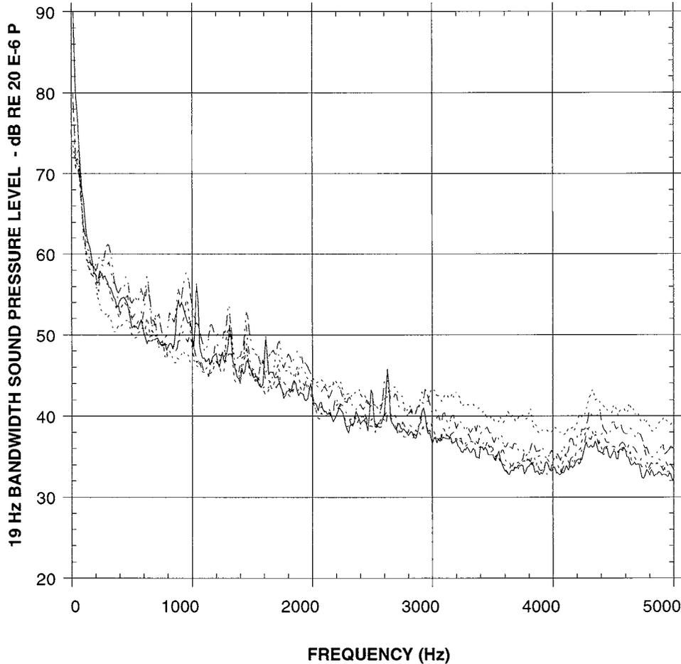
Figure 18. Fourier spectrum of wayside noise at the high rail side for four samples of Car No. 9 with treated Bochum 84 wheels.
