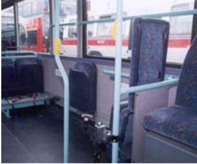
FIGURE 14 Combi system of forward and rear facing in one location, 10.6-m (35-ft) BC Transit low-floor bus (future standard for all buses).
