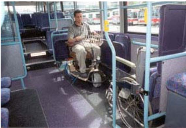
FIGURE 17 Combi 2 design for two travelers in the same position on BC Transit bus.
