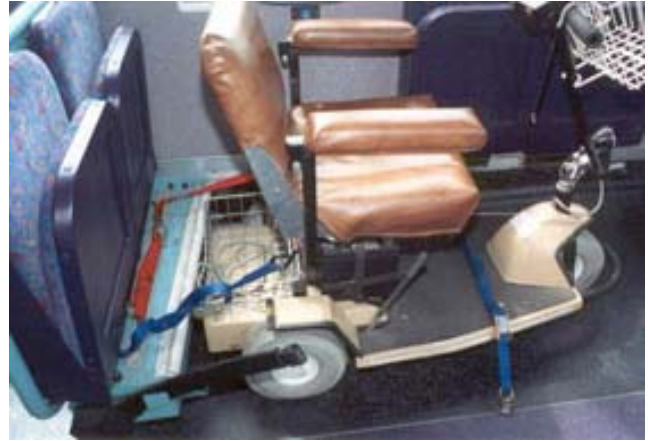
FIGURE 11 Forward-facing position in combi design, with two rear tie-downs and one strap over the footrest of the scooter.
