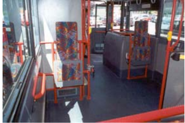
FIGURE 18 Double-decker BC Transit low-floor bus: Combi system roadside, one rear-facing system curbside.
