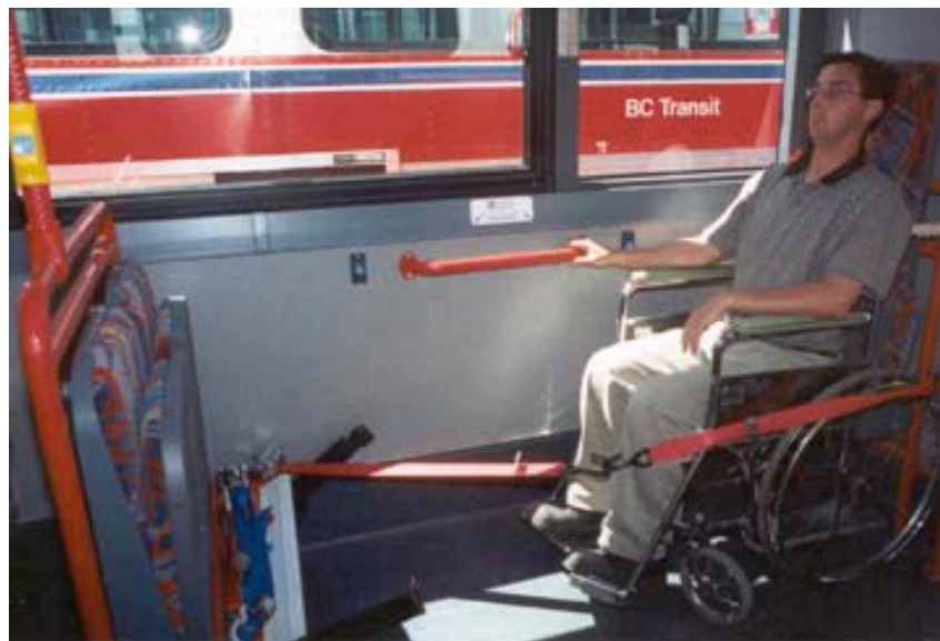
FIGURE 15 Combi 1 design on BC Transit double-decker bus with front- and rear-facing design in same position, and hooked straps to prevent tipping.
