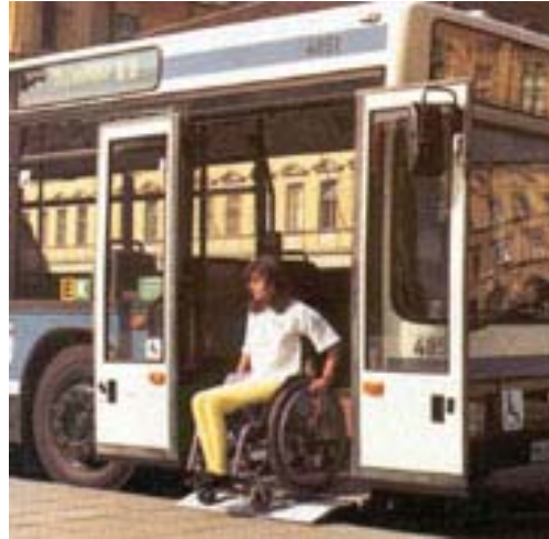
FIGURE 9 Access over ramp at front door (Germany).
