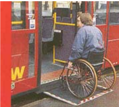
FIGURE 8 Access over ramp at center door (United Kingdom).
