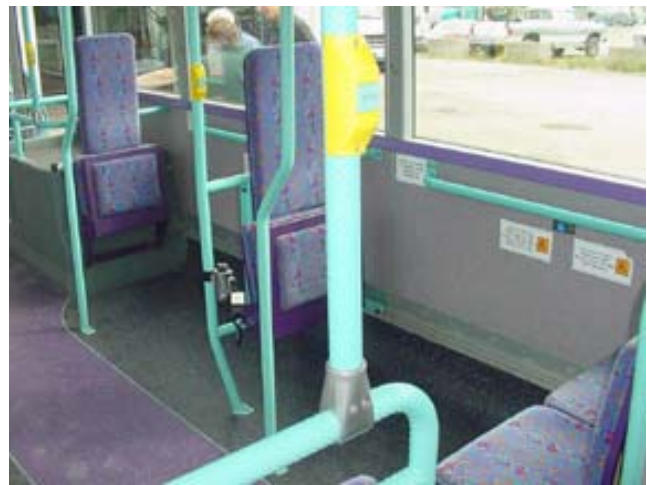
FIGURE 13 Two rear-facing systems in tandem at curbside in 9-m (30-ft) BC Transit low-floor bus.
